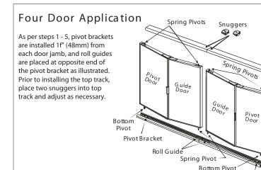
bracket screw and slide pivot bracket along track, once located, re-tighten screw. Height adjustment is achieved by turning the adjustment bolt with a Phillips screwdriver as shown. Attach the door pull onto the pivot panel at desired height (approx. 40" (1016mm) from the floor). Clean the stile with isopropyl (rubbing) alcohol before attaching the pull to the panel as this maintains proper adhesion. Locate and tighten snugger with
