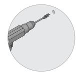
**A)** Drill the hole locations requiring a wall anchor with a 3/4" spade bit.
