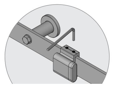
**A)** Move the door to the closed position (**Step 17-B** opposite side) and slide the other appropriate end stop onto the end of the track until it contacts the hanger strap and tighten the set screws on top.
