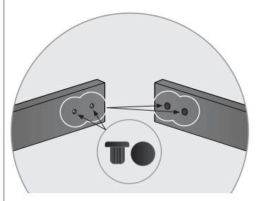
**A)** To finish the installation attach the Barn Door Track Joiner Plugs to both ends of the Track.
