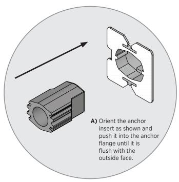
**Note:** Prior to inserting the Anchor Insert, ensure there is NO drywall paper or debris covering or inside the threaded anchor plate, so the bolt will thread easily.
