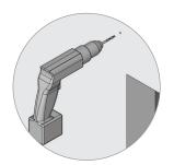
A) Drill the hole locations going into a wood stud or header with a 7/32" drill bit to a depth of appx. 1 ½ inch.
