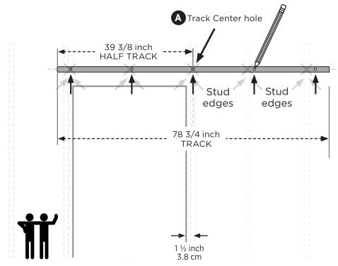
A) Using the track as a template, position the tracks center hole over the drawn horizontal line's center "x" mark (Step 5-C).
