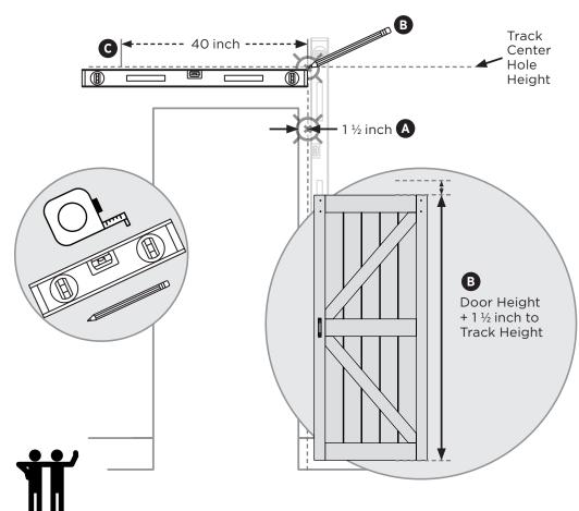
A) Once you determine which side of the opening your door will open to, Measure 1½ inch (3.8 cm) to the right and mark your center point then draw a light vertical line (roughly) 6 inch upward past the door opening (this determines the vertical center of the Track).
