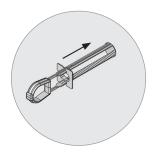
A) Keep the pull ring vertical and pull the anchor back so the steel anchor plate sits vertically against the inside face of the drywall.
