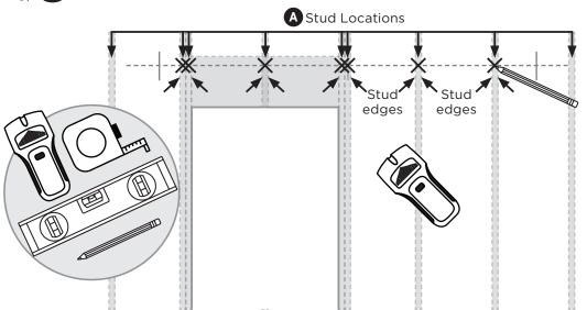
A) Use a stud finder to locate and mark the center and edges of each stud and cripple, as well as the top of the door header to ensure it is at least 1 inch above the line drawn.
