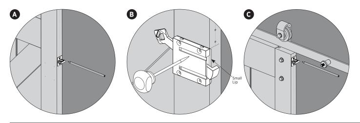
A) Using a 1/8" drill bit, drill all the marked hole locations <sup>3</sup>/<sub>4</sub>" deep, including the front door assembly holes.
