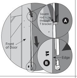
A) Insert the engagement pin block assembly into the bottom end of the rod, with the pin facing the side of the door the handle will be affixed to (as shown in step 8).
