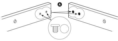
A) To finish the installation attach the Barn Door Track Joiner Plugs to both ends of the Track
